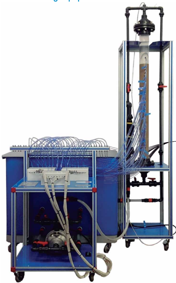
① Unit: EFLPC. Deep Bed Filter Unit
