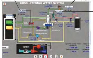
HUB II screen 2.9. Real time simulation of the Heat Recovery feeding water system control loops
