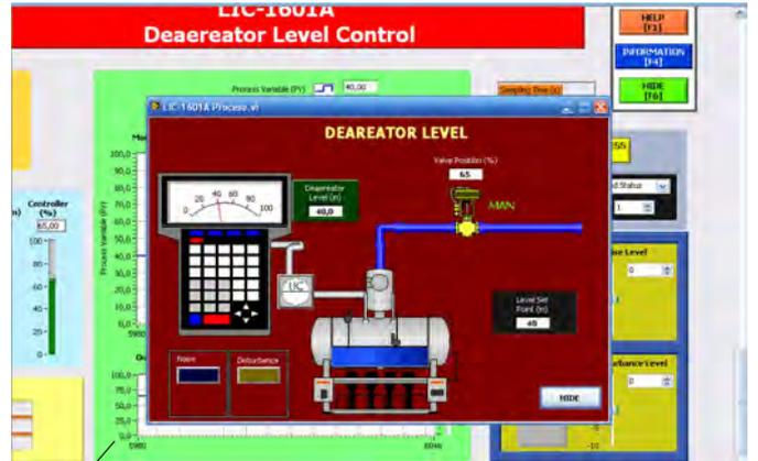
HUB II screen 2.9.2. Real time simulation of the local control loop of deaerator level (LIC-1601A)
