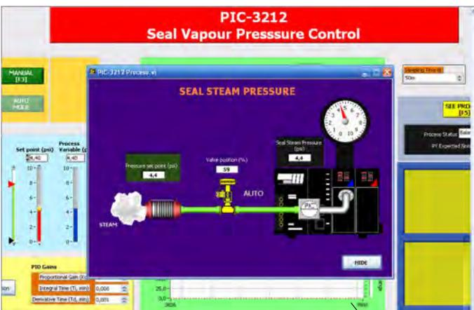
HUB II screen 2.6.1. Real time simulation of the local control loop of seal steam pressure (PIC-3212)
