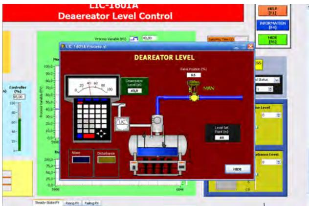
HUB II screen 2.8.1. Real time simulation of the local control loop of deareator level (LIC-1601A)
