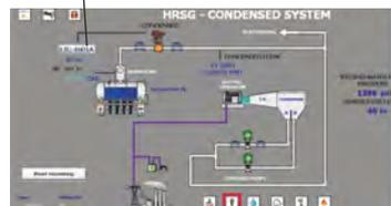
HUB II screen 2.8. Real time simulation of the Heat Recovery condensed system control loops
