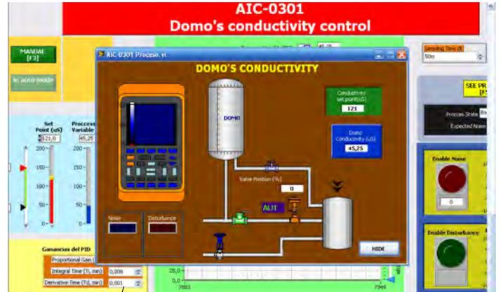
HUB II screen 2.11.2. Real time simulation of the local control loop of domo's conductivity (AIC-0301)
