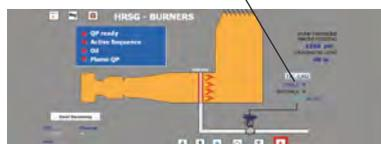
HUB II screen 2.12. Real time simulation of the Heat Recovery burners control loops
