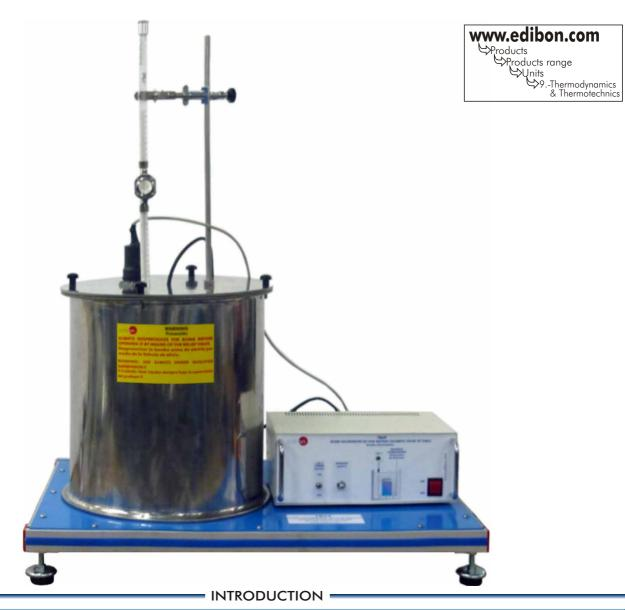
Calorimetry is a fundamental test of great significance to anyone concerned with the production or utilization of solid or liquid fuels.
