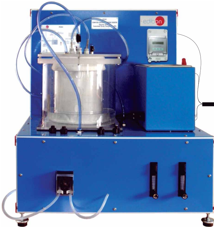
① Unit: PDAC. Aerobic Digester
