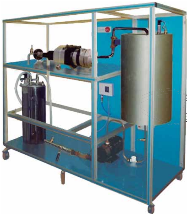
① Unit: TORC. Organic Rankine Cycle Unit
