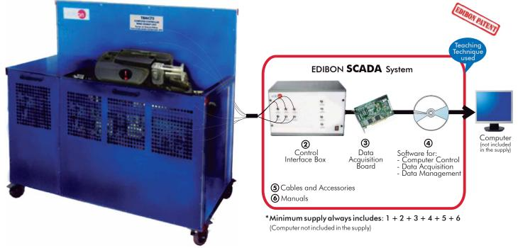
1 Unit: TBMC75. Test Bench for Four-Cylinders Engines, 75 kW
