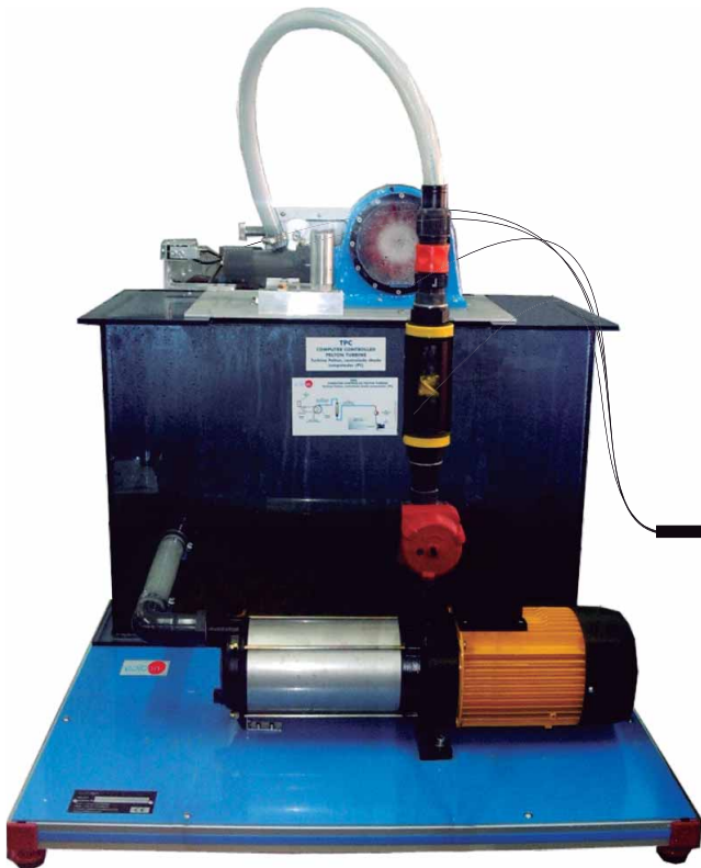
① Unit: TPC. Pelton Turbine
