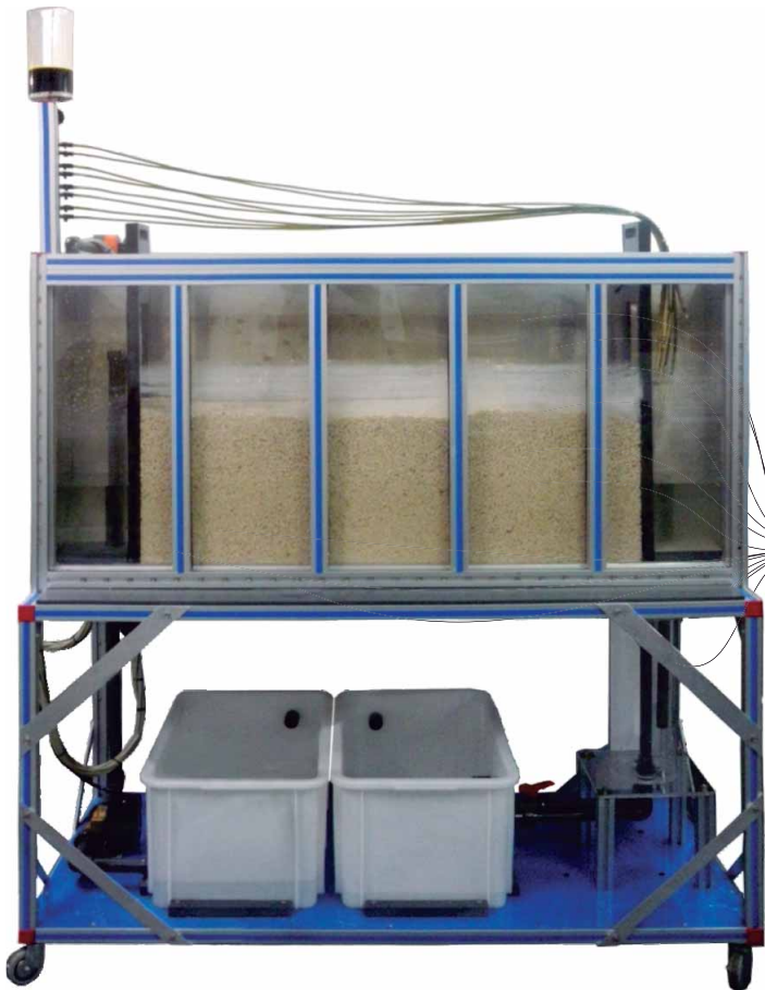
① Unit: PDFDC. Drainage and Seepage Tank
