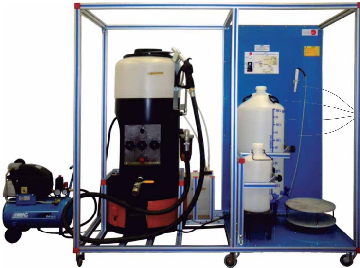
① Unit: EBDC. Biodiesel Process Unit
