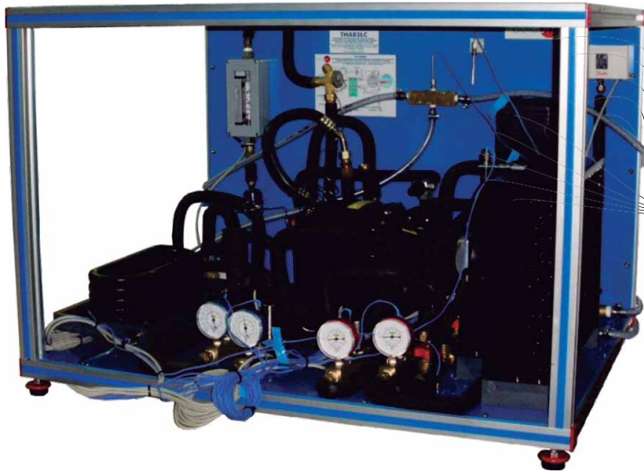
① Unit: THAR2LC. Refrigeration and Air Conditioning Unit (two condensers (water and air) and one evaporator (water))
