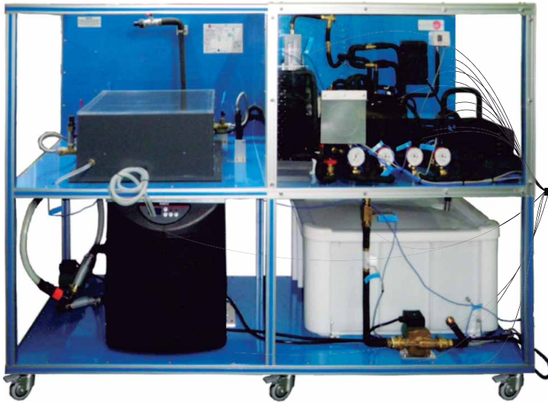
① Unit: EG5C. Geothermal (low enthalpy) Energy Unit
