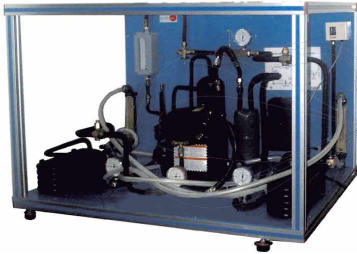
① Unit: THBLLC. Heat Pump Unit (one condenser (water) and one evaporator (water))
