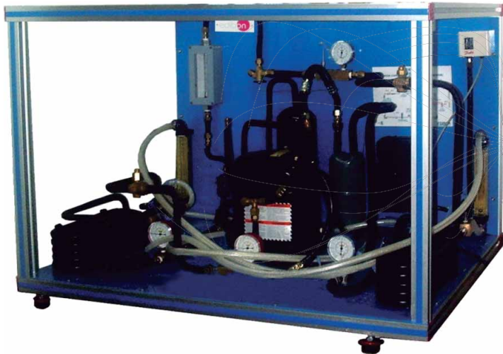
① Unit: THARLLC. Refrigeration and Air Conditioning Unit (one condenser (water) and one evaporator (water))
