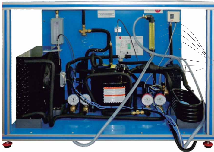
① Unit: THARALC. Refrigeration and Air Conditioning Unit (one condenser (air) and one evaporator (water))
