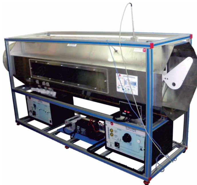
① Unit: EEEEC. Wind Energy Unit
