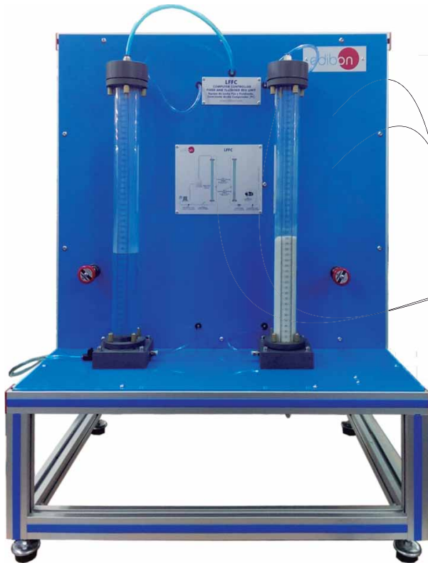
① Unit: LFFC. Fixed and Fluidised Bed Unit
